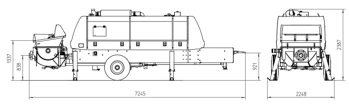
Note: Standard version BSA 2110 HP D. Dimensions and weights depend on equipment. Subject to technical modifications and errors.
