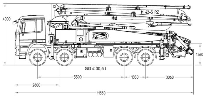
Note: Standard version. Dimensions and weights depend on truck, pump model and equipment. Dimensions in mm, MB-Actros 3241, Euro 5 as example.
