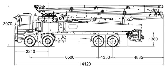
Note: Standard version. Dimensions and weights depend on truck, pump model and equipment. Dimensions in mm, MB-Actros 4640 B, Euro 2.
