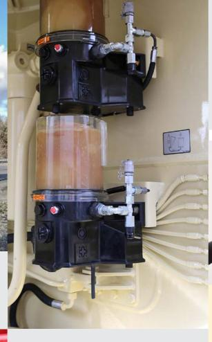
Combined centralized lubrication system: The electrical centralized lubrication system for hopper, A-hinge and four-point bearing ensures that the service life of the components that are subject to high stress is maximized without any additional work or expense. The optional centralized lubrication system on the boom means that the daily inspection process can be further streamlined. Time equals money.
