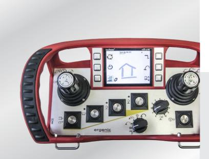
All possible displays and settings can be read optimally on the large, high-resolution colour display – EGD-RC (Ergonic® Graphic Display Remote Control).
