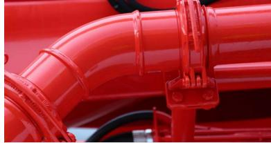
Maintenance-free components reduce operating and maintenance costs, for example thanks to wear-optimized standard elbows with long joins for maximum delivery line service life.
