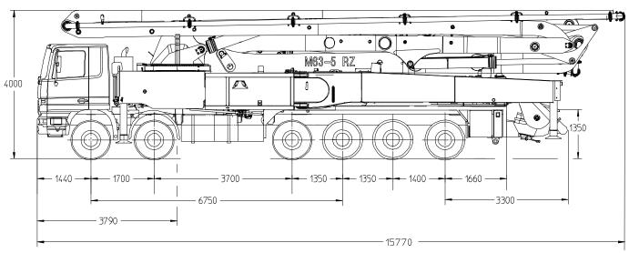
Note: Serial version. Dimensions and weights depend on truck, pump model and equipment. Dimensions in mm, MB-Actros 6560 as example
