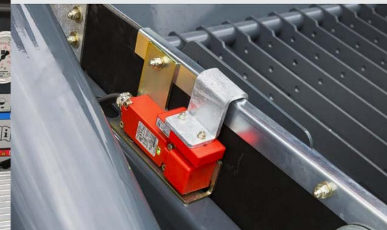
**Agitator safety shutdown via RFID** (Radio Frequency Identification): A detection system using electromagnetic waves, including start-up protection, ensures optimum safety for machine operators.
