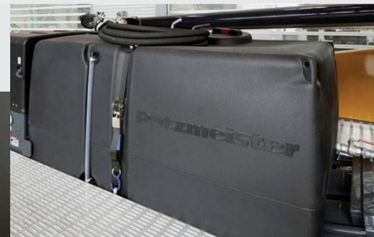
**Large water tank** enables you to avoid having to fill up on a regular basis and therefore reduces working time. It also offers a large reserve for cleaning operations.
