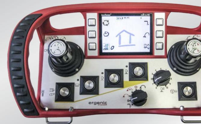
All possible displays and settings can be read optimally on the large, high-resolution colour display – EGD-RC (Ergonic® Graphic Display Remote Control).
